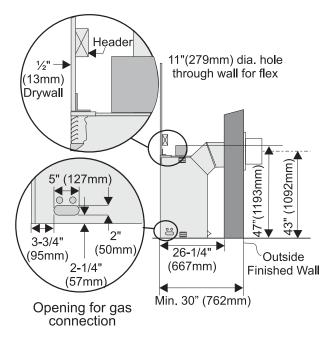
Note: 43" (1092mm) is the minimum height for flex termination and Simpson Dura-Vent terminations.
